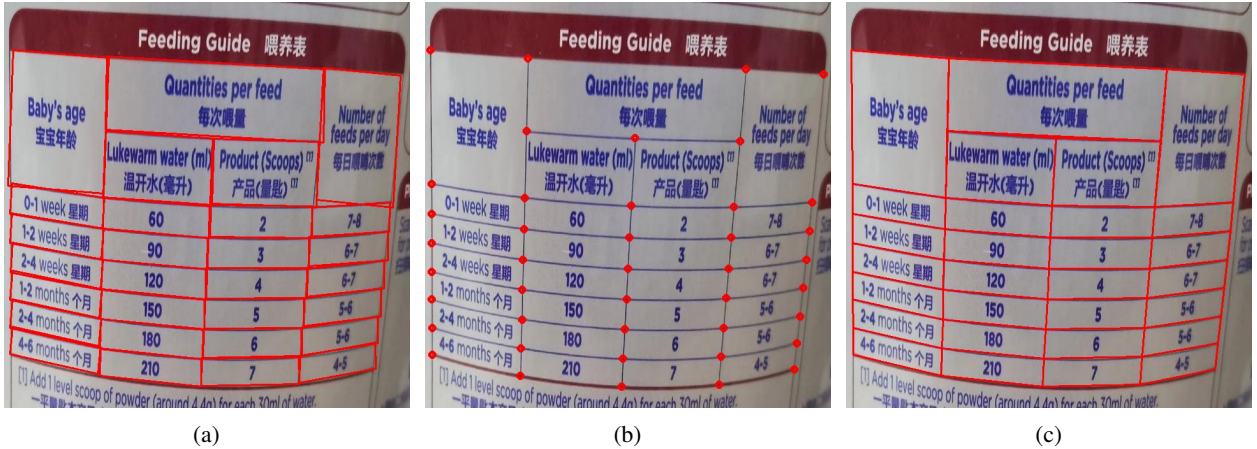
Figure 4: Visualization of cell spatial location alignment. (a) is the result of cell spatial location regression, (b) is the result of cell corner point detection, and (c) is the result after cell spatial location alignment.
