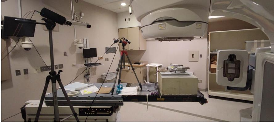
Fig. 1: The camera setup with both cameras positioned as high as possible to minimize the angle between the camera-isocenter axis and the central axis of the beam. The C-blue and Basler cameras were positioned next to and on top of the treatment couch, respectively.
