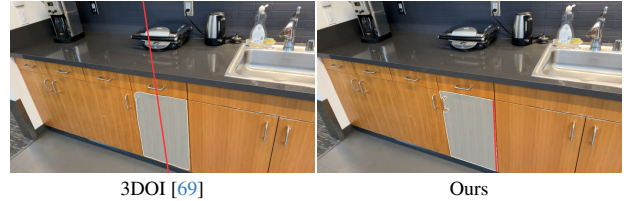
Figure 4. Articulation Estimation: We visualize the estimated revolute axes and articulated object masks produced by 3DOI [69] and DRAWER, demonstrating that DRAWER achieves more precise articulation estimation due to its underlying 3D geometry.
