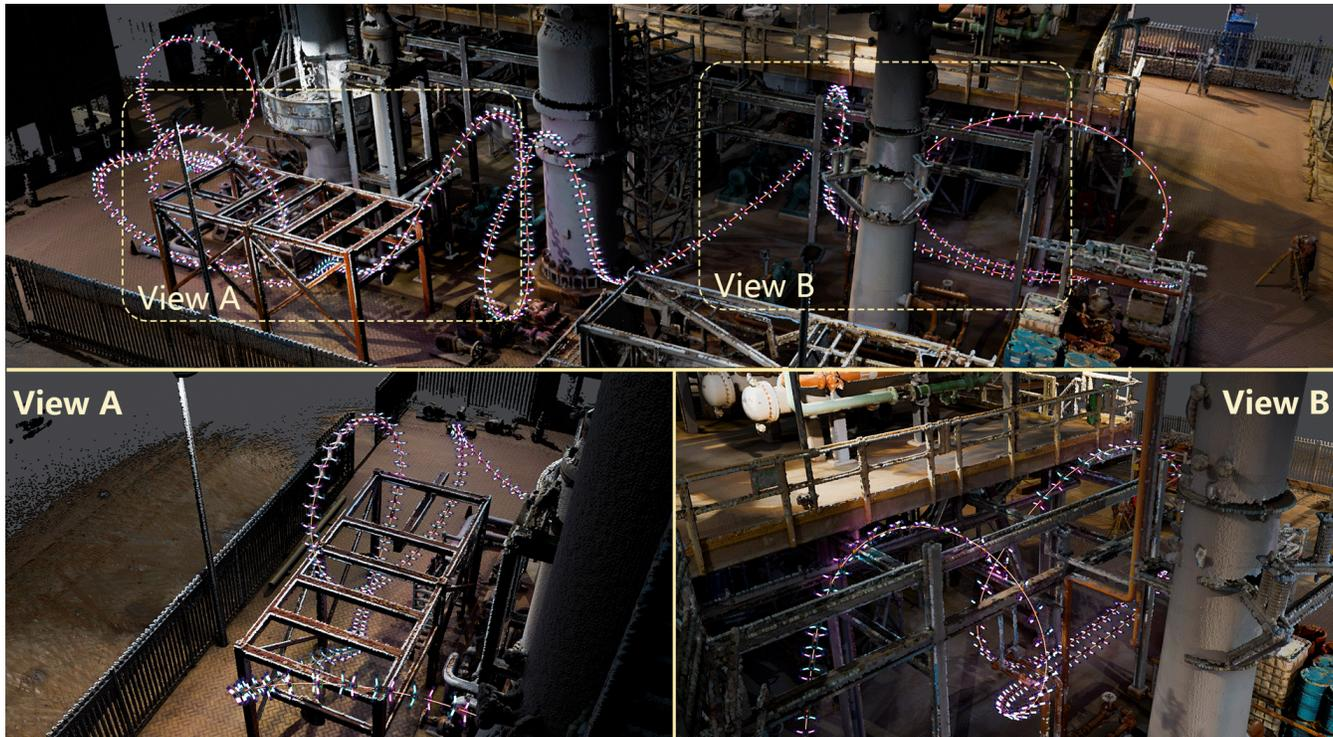
Fig. 1: Our method enables automatic generation of successive long-horizon aerobatic maneuvers, allowing drones to traverse through a complex industrial factory with dynamically feasible motion.
